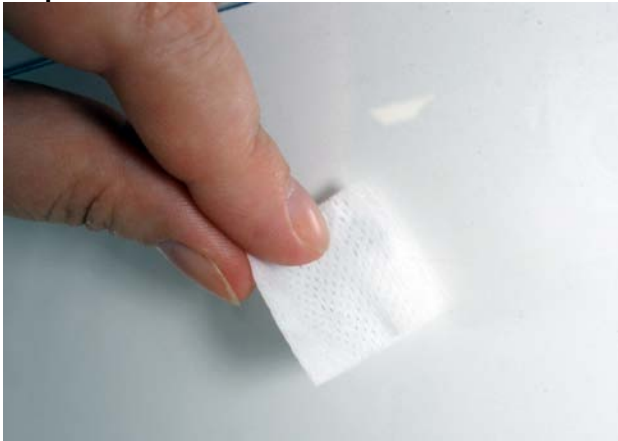
Figure 14. Adhesive Mount Antenna – Step 2. Peel Protection from Adhesive Strip
