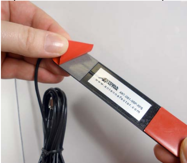
Figure 14. Adhesive Mount Antenna – Step 2. Peel Protection from Adhesive Strip
